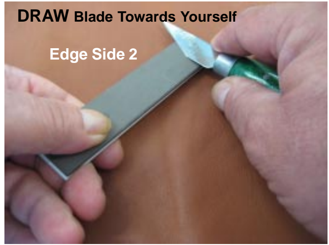
Step 4 - Hold the knife at a steady angle and DRAW it TOWARDS yourself, on a DIAGONAL path.
